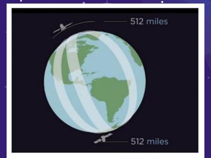
The picture above shows Suomi NPP and NOAA-20, the two satellites in the Joint Polar Satellite System in their polar orbit. Each satellite is approximately 512 miles above Earth's surface, traveling at approximately 17,000 miles per hour. At this speed, JPSS completes 14 polar orbits in one day, covering the entire Earth twice a day.
